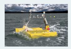
Harnessing ocean waves to power remote marine applications
