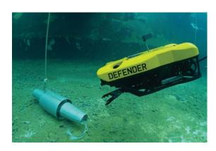
VideoRay tethered, underwater Remotely Operated Vehicles (ROVs) are used for today's toughest aquatic missions, from mine countermeasures to port security and surveillance.
