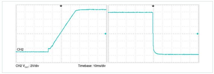
Figure 4 — Rise and fall, +12V output, nominal line, nominal load, enable/disable
