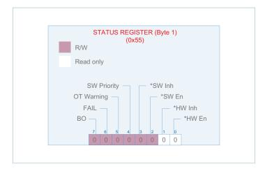
Under some conditions, it is desirable to ignore potentially damaging conditions. For this purpose the power supply provides a battle override function in the system status register. If bit 7 in the status register is set, then any non-recoverable events that would normally shut down the supply will not do so.
