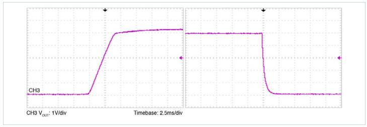
Figure 6 — Rise and fall, +5V output, nominal line, nominal load, enable/disable
