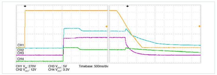
Figure 1 — Turn-on and turn-off characteristics at nominal line and nominal load, to main outputs
