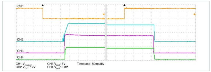
Figure 2 — Turn-on and turn-off time from enable to outputs
