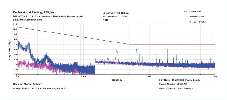
Figure 11 — Conducted emissions of power return at full load
