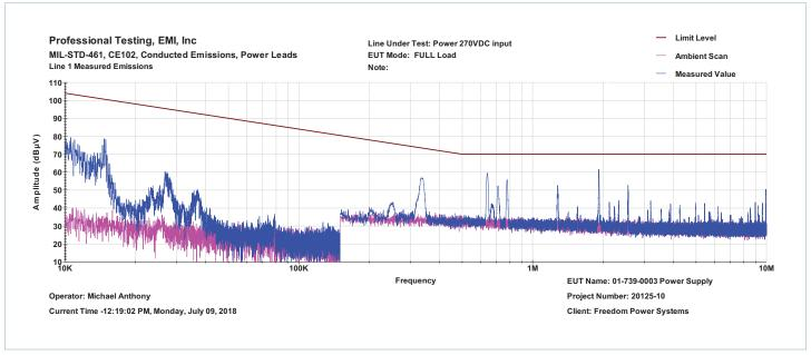
**Figure 10** — Conducted emissions of 270V<sub>DC</sub> input at full load
