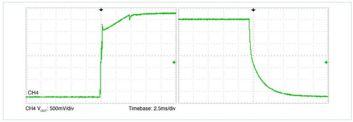
Figure 8 — Rise and fall, +3.3V output, nominal line, nominal load, enable/disable
