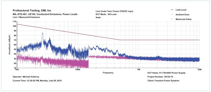
Figure 12 — Conducted emissions of 270V<sub>DC</sub> input at no load
