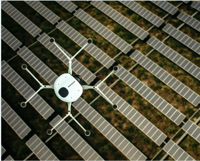
Example of solar panel inspection (Source: Doosan Mobility Innovation)
