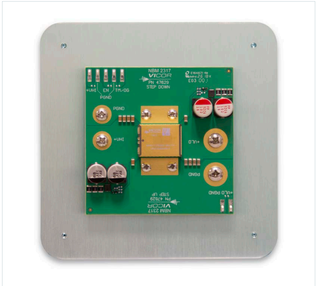
Figure 6 NBM™ evaluation board mounted on coldplate
