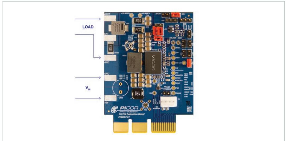
Install: J301, JTRK, JISP and JISN to connect IS+ and IS- to ground.
