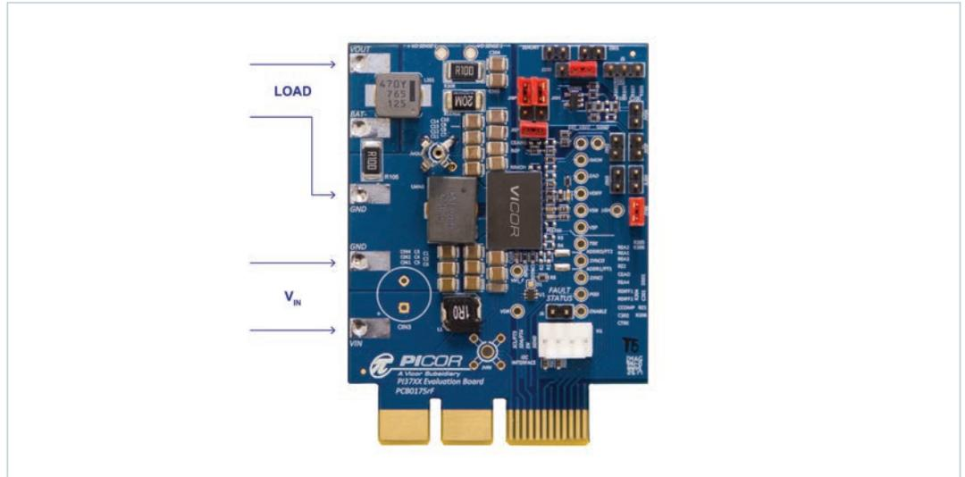
Install: J1SP, J1SN connecting  $R_{SENSE}$  to IS+ and IS-, J200 connecting  $I_{MON}$  to LGH, JTRK.
