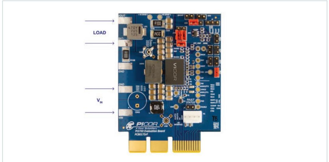
Install: J200 connecting R106 to R205/R206, JTRK, JISP and JISN shorting IS+ and IS- to ground.
