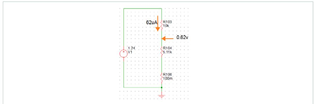
The charging current can be adjusted by changing R104 per the following equation.
